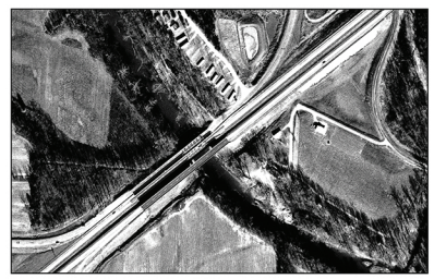
This pre-interstate aerial of US 66 from 1967 shows the new eastbound bridge and the annexed existing westbound bridge for the 4-lane alignment.
