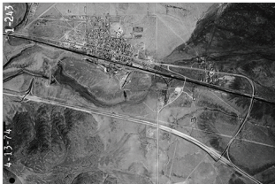
State of I-40 at Seligman in 1974. All traffic was directed through town from Exit 123 (right side of photo) until the bypass was completed in 1978. Note that Exit 121 (left side of photo) was only partially built.
